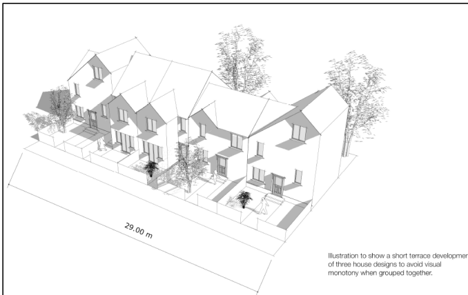
Figure 45: showing how the effects of a longer building facade can be managed
