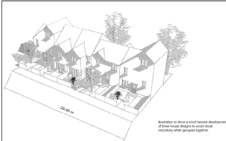
Figure 34: showing how the effects of a longer building facade can be managed
